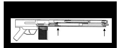
This figure illustrates the placement of the front and rear gas ports for the dual-stroke firearm design.
